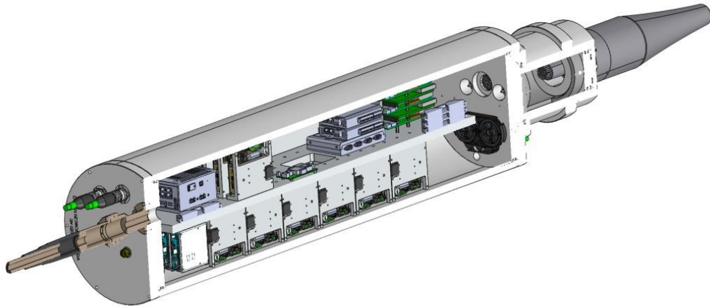
Mooring junction box
