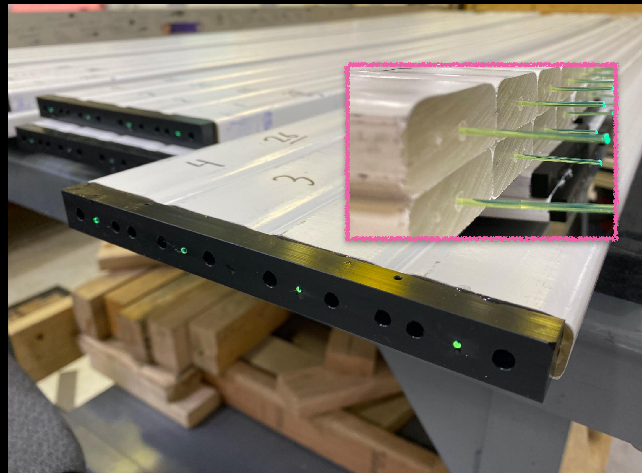
Hadronic calorimeter scintillator bars layer
