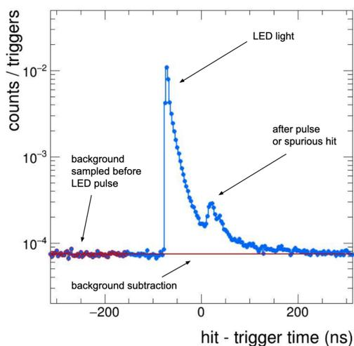
Figure 4. Signal from 1 p.e. and after-pulse
