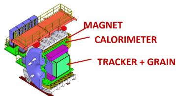
re-use/upgrade KLOE (LNF): 0.6 T superconduction solenoid magnet 4pi electromagnetic calorimeter new design: internal straw tube tracker GRAIN LAr Meniscus (1 T) LNS involved in both activities
