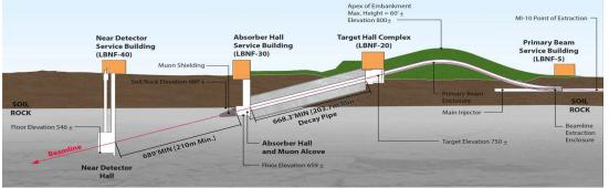
5.8° inclined beam (specially created 18 m artificial hill)
