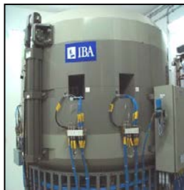
Cyclotron for the Radiotracer production
