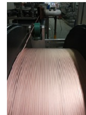
copper plated Ti- MgB_2 tape
