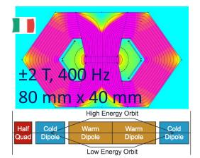
Combination of DC SC magnets (10 T) and AC resistive magnets (± 2T)
