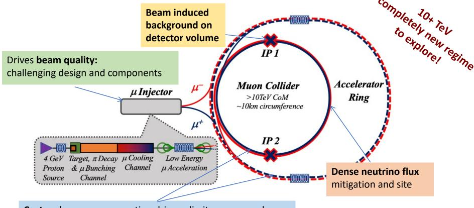
**Cost** and **power** consumption drivers, limit energy reach e.g. 30 km accelerator for 10/14 TeV, 10/14 km collider ring
