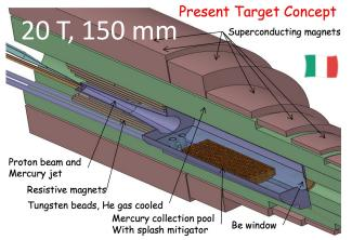
High-field and large aperture target solenoid with heavy shielding to withstand heat (100 kW/m) and radiation loads
