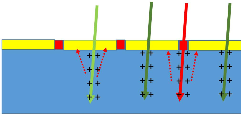
If a particles is detected in a region between two strips the charge generated by the particle can be shared between the two strips – **This is an INTERSTRIP event**
