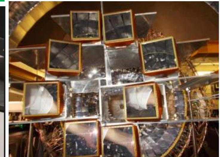
I will show results of a test experiment with the **reaction  $\alpha+^{12}\text{C}$  at 64 MeV performed at LNS** – 4 FARCOS telescopes were used mounted at 40 cm from the target. We will show the coincidence measurements of 2-3  $\alpha$  particles to test the pixellation work
