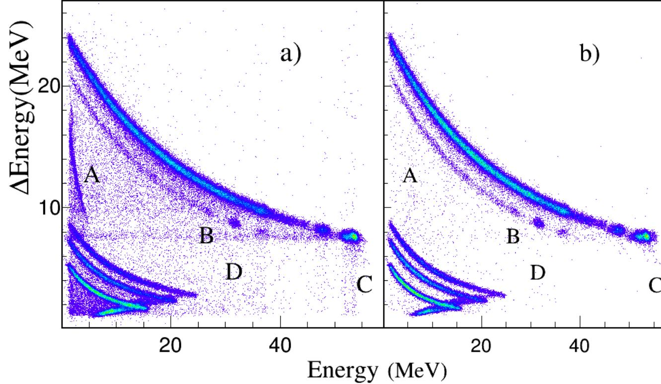
Near guard ring events induce strange signals with fast decay time in the strips 0 and 31
