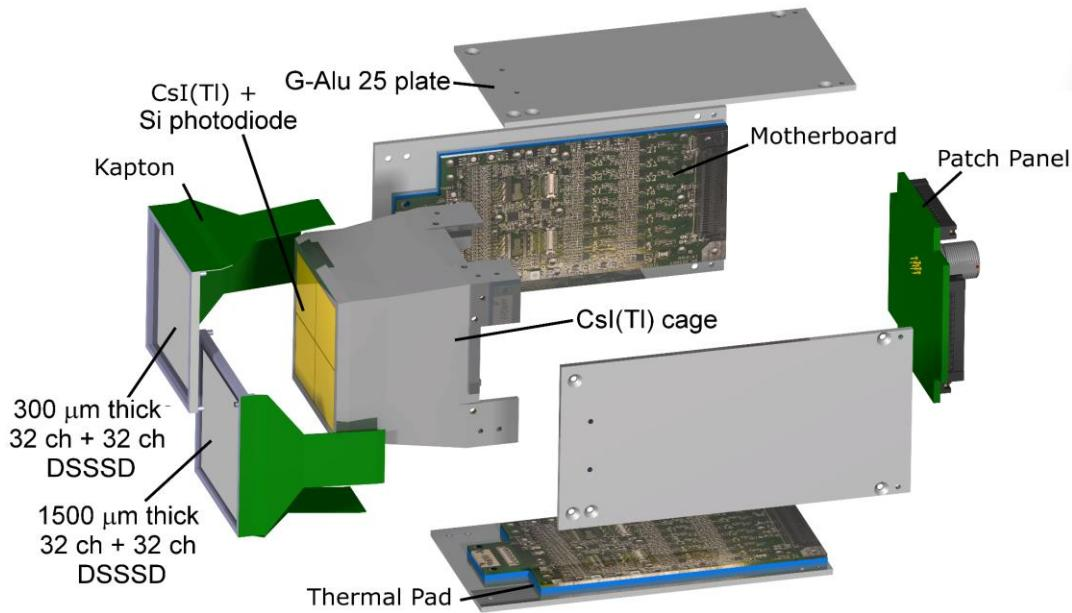
Farcos is an array of 20 triple telescope with two stages of DSSSD 300  $\mu\text{m}$  and 1500  $\mu\text{m}$  both with 32x32 strips 2 mm wide with a third stage with 4 Csl(Tl) 6 cm long
