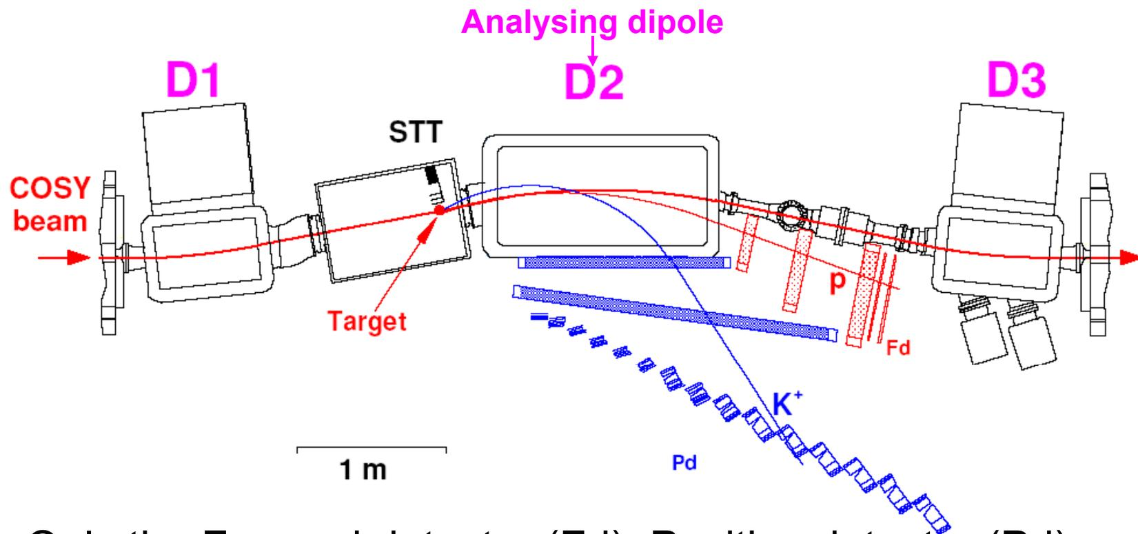
Only the Forward detector (Fd), Positive detector (Pd) and the silicon tracking telescope (STT) were used in experiments at 1.83, 1.92, 2.02, and 2.65 GeV.
