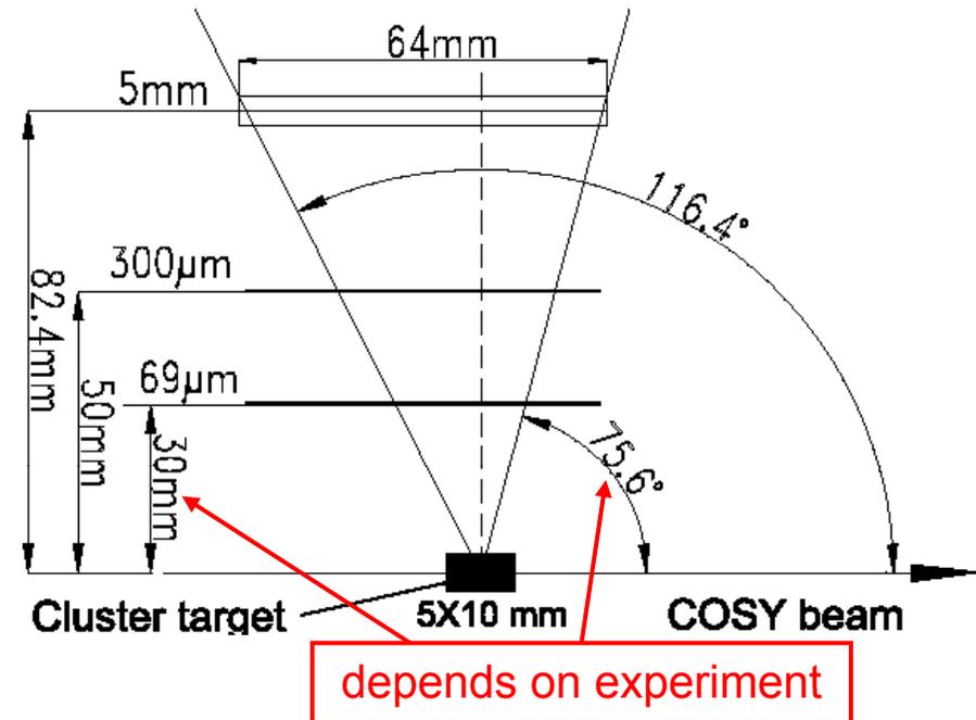
Telescope arrangement of three double-sided silicon strip detectors:
