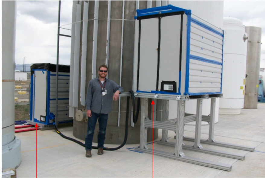
1.2 m x 1.2 m drift tube gas trackers X-Y measurement
