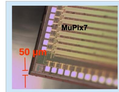
Monolithic pixel sensor in 180 nm HV-CMOS
