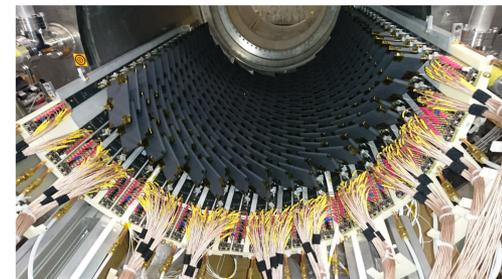
light drift chamber in a magnetic field
