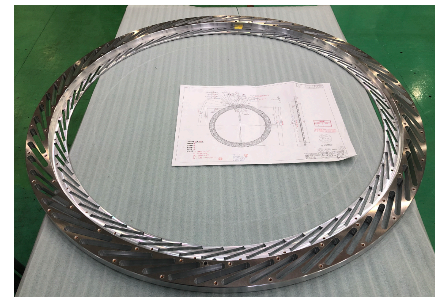
CTH Counter supporting structure
