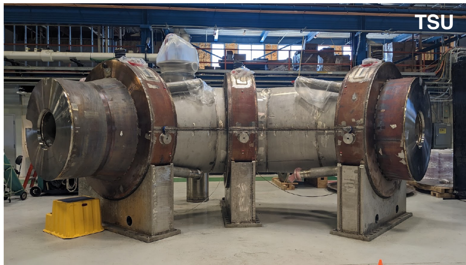
PS cold mass – inner shield dry run insertion
