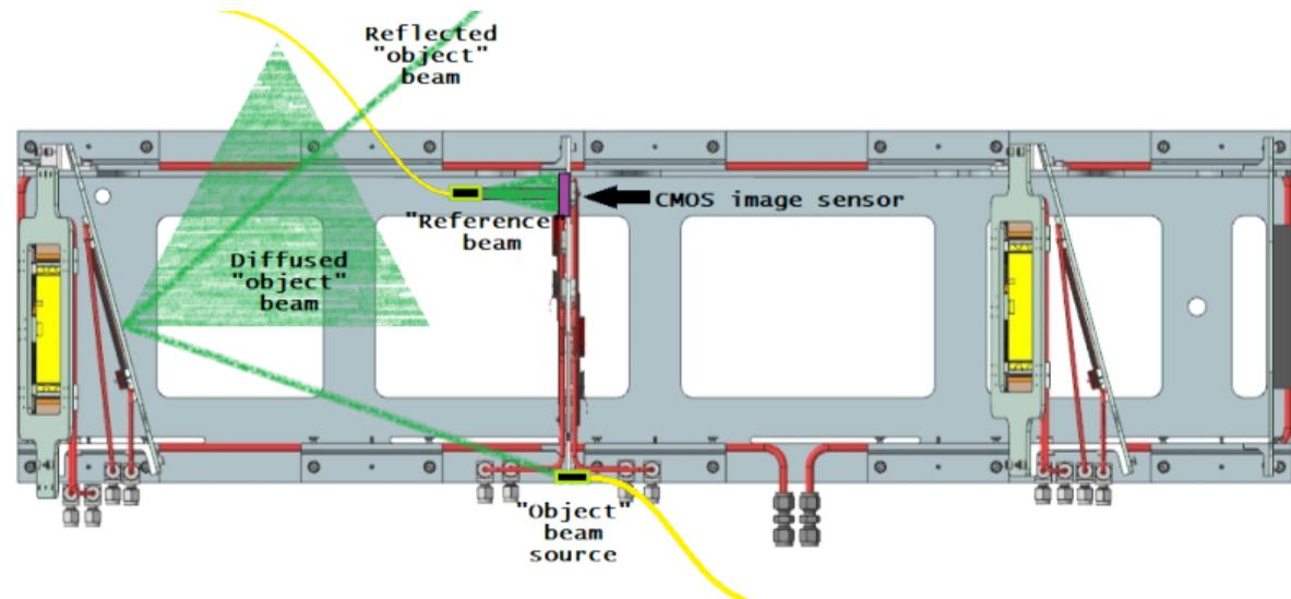
Time-dependent interferometry by digital superposition of raw holographic images taken at different time  $t$ . Sensors must be off for HAM DAQ.
