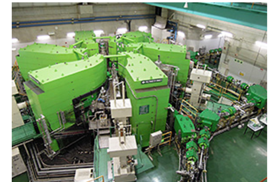
Ring Cyclotron \sim 392 \text{ MeV} (variable) 1.1 \mu\text{A} proton, (0.4kW)
