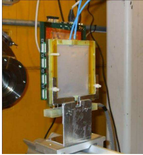
Figure 1: Front view of the nGEM detector installed on the Vesuvio beam line.
