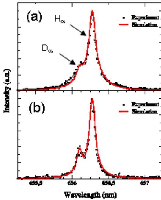
LIBS spectra ( $H_{\alpha}$  and  $D_{\alpha}$ ) of a carbon fiber composite tile of Tore Supra fusion reactor with 500 ns (a) and 1000 ns (b) [4]. The intensity ratio difference in recording is attributed to diffusion of lighter H-atoms out of the plume.
