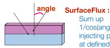
Sum up 1/cos(angle) of injecting particles at defined surface
