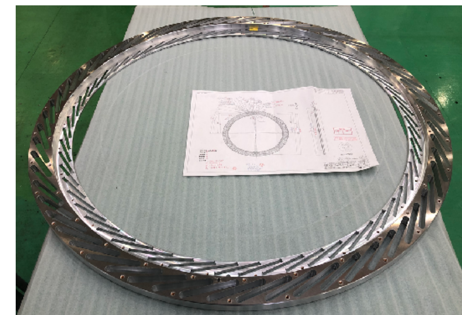
CTH Counter supporting structure
