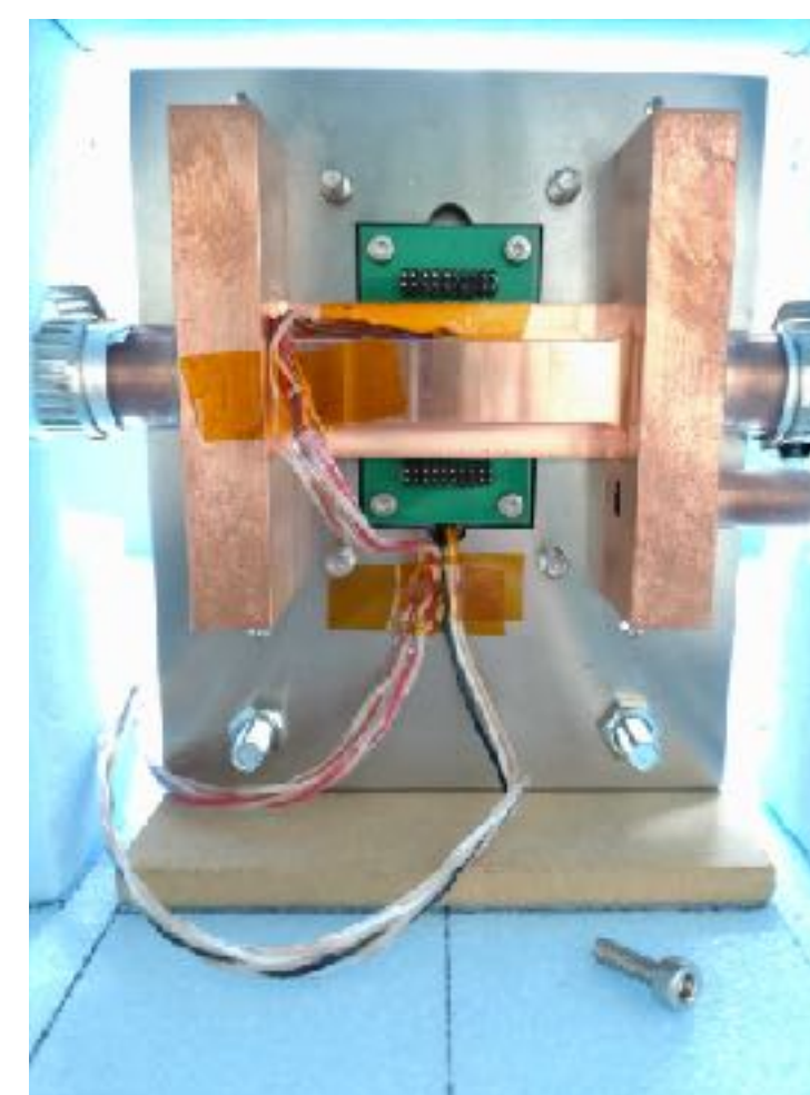
MPPC cooling system to achieve \sim -40^\circ\text{C}
