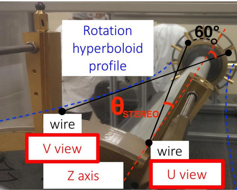
Stereo wire geometry for longitudinal hit localization
