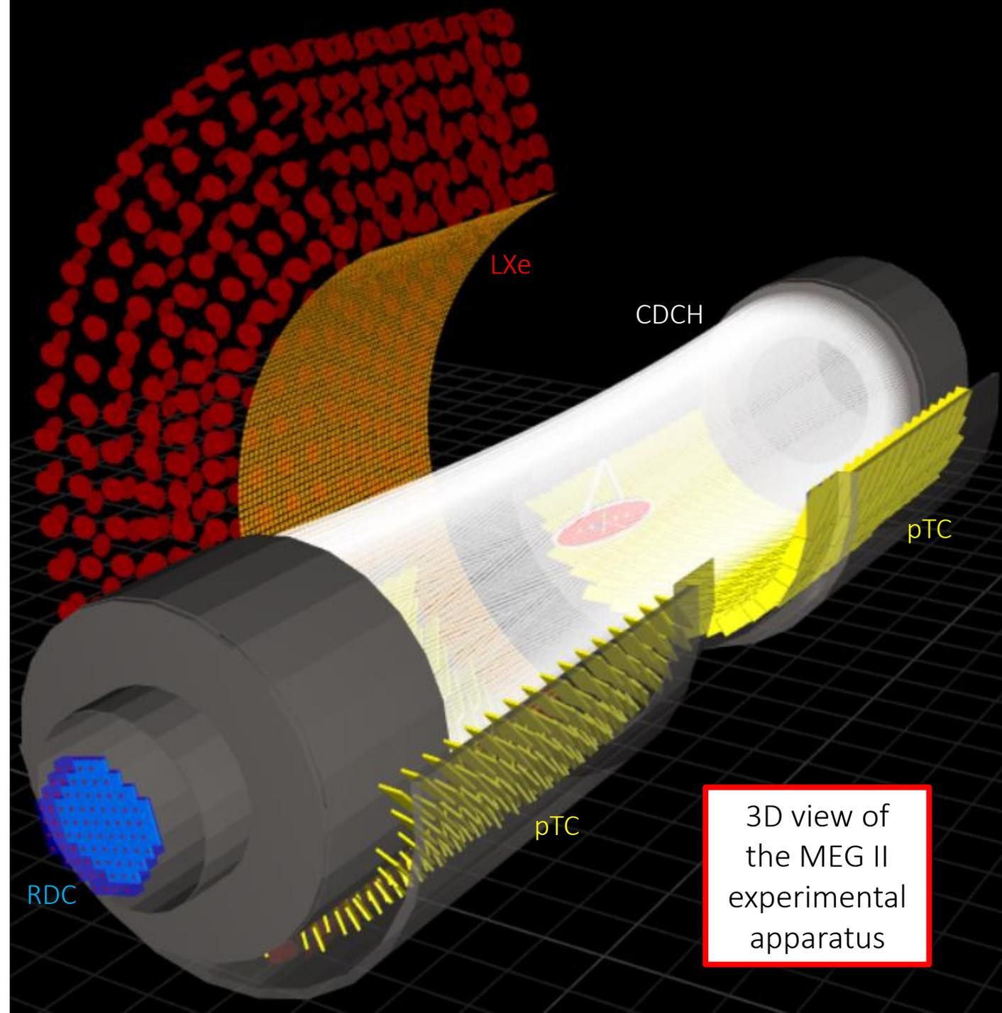
3D view of the MEG II experimental apparatus
