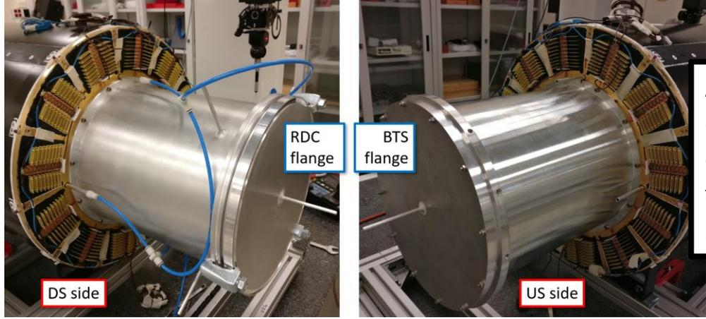
Aluminum inner extensions to connect CDCH to the MEG II beam line
