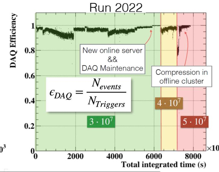
Significant improvement in the DAQ efficiency and stable operation up to 30 Hz trigger rate (× 3 the design)
