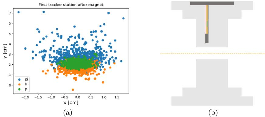
Fig. 2.: (a) Hit distribution of the  $\Lambda_c$  daughters in the first tracking station. (b) Schematic drawing on the inner boxes of the roman pot, one filled with the VeloPix sensors.
