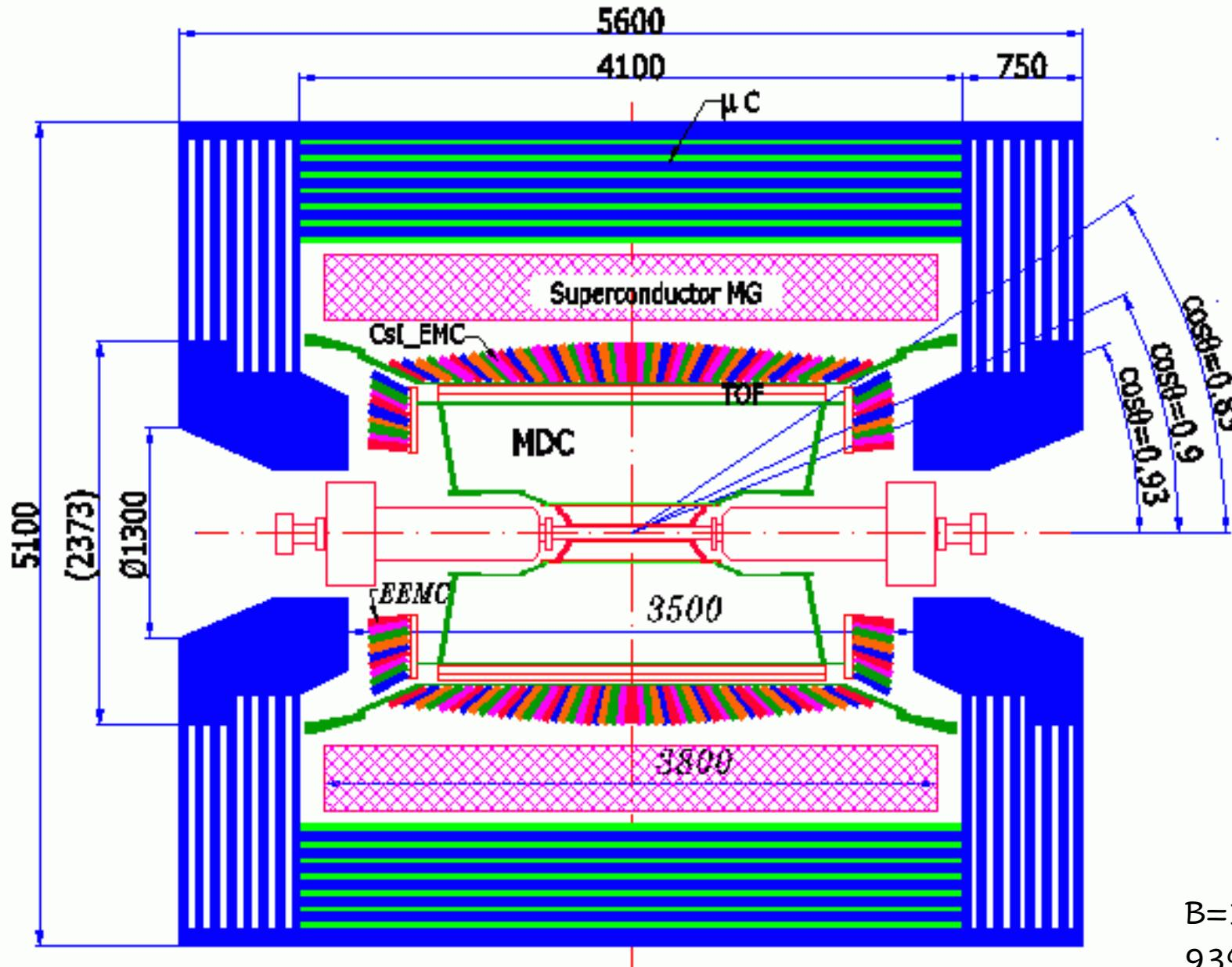
**MDC:** main drift chamber (He 60%,propane 40%)  $\sigma(p)/p < 0.5\% @1\text{ GeV}$ ,  $\sigma(xy) = 130\text{ mm}$ , 6%  $dE/dx$
