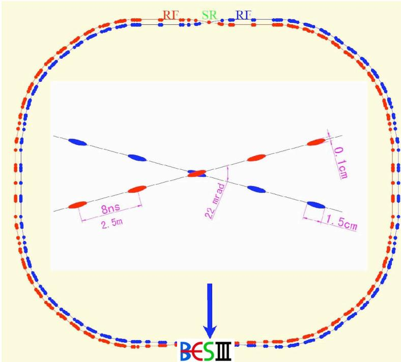
Double ring electron-positron collider, operated @ IHEP
