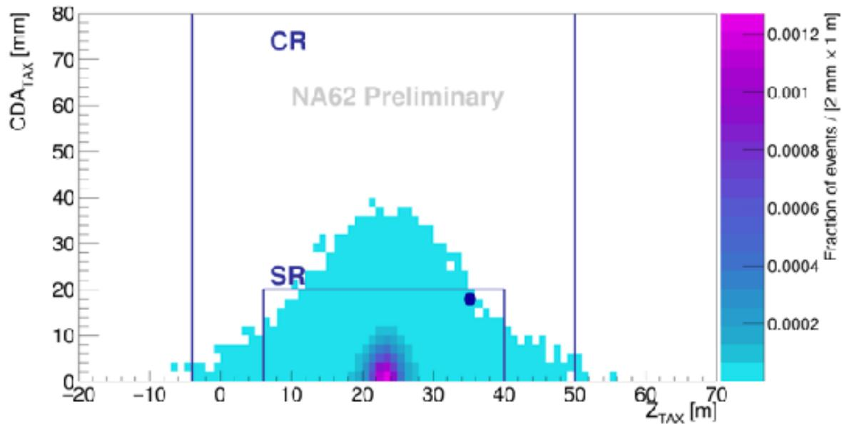
$Z_{\text{TAX}}$  → longitudinal position of the primary vertex,  $\sigma_z \sim 5.5$  m
