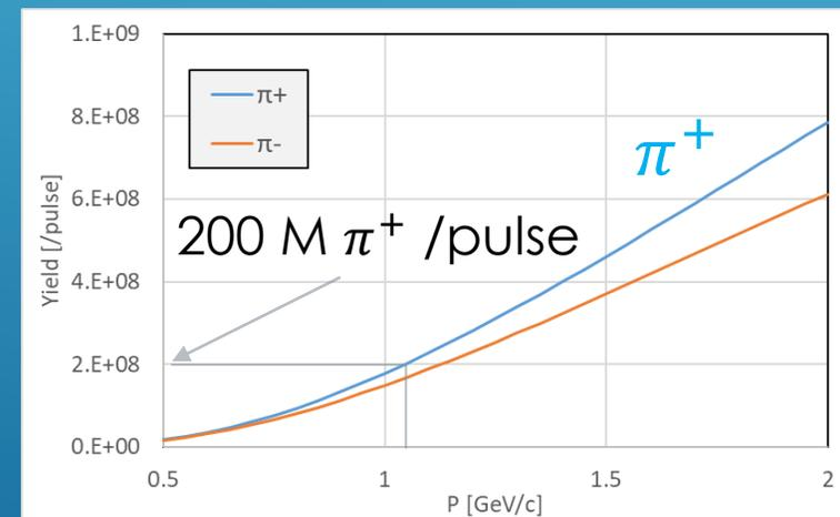
3deg. Ext. angle,  $5.0 \times 10^{13}$  ppp on 50% loss target (T2) 46kW, 5.2s (92kW on T1)
