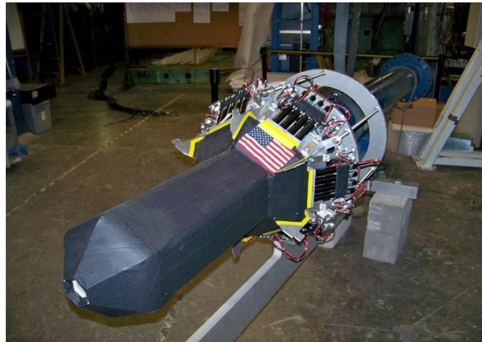
*Photo of the start counter during CLAS's construction.*
