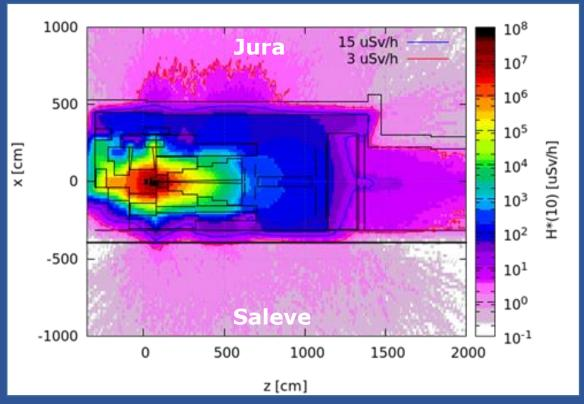
A massive shielding around the absorber region, where the beam will be dumped, has been designed
