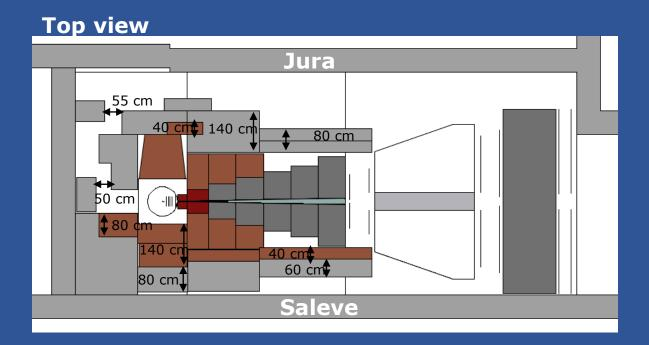
A massive shielding around the absorber region, where the beam will be dumped, has been designed
