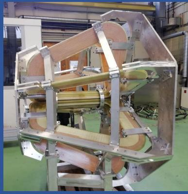
□ A prototype (1:5 scale) was built and tested in 2020-2021 by the CERN-EP-DT group, to check calculations and investigate mechanical solutions, in view of the final object  Measurements of resistance, inductance, cooling performance and magnetic field were carried out
