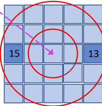
Due to the TIR, photons only hit the PC in a radial band ~[5.5 .. 12.0] mm
