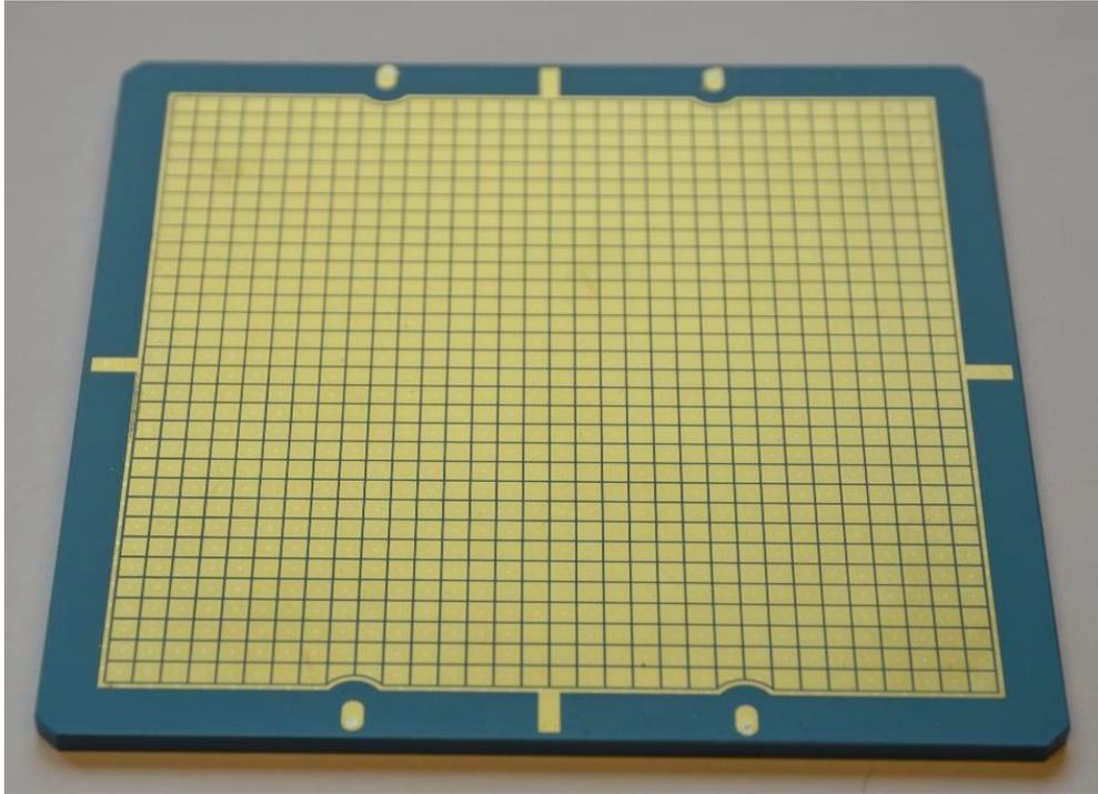
HRPPD anode plate with a non-trivial internal trace routing
