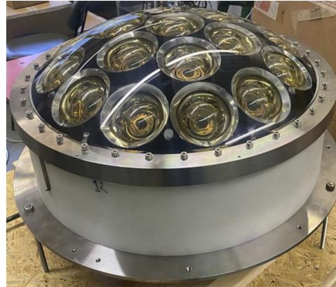
~3600 8 cm OD PMTs with wavelength shifting plates.
