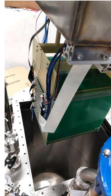
Insertion into cryostat
