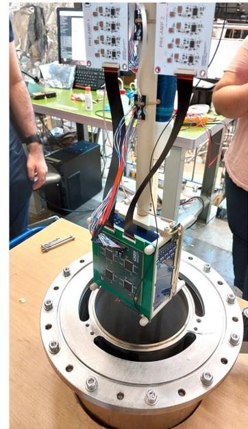
Insertion into cryostat
