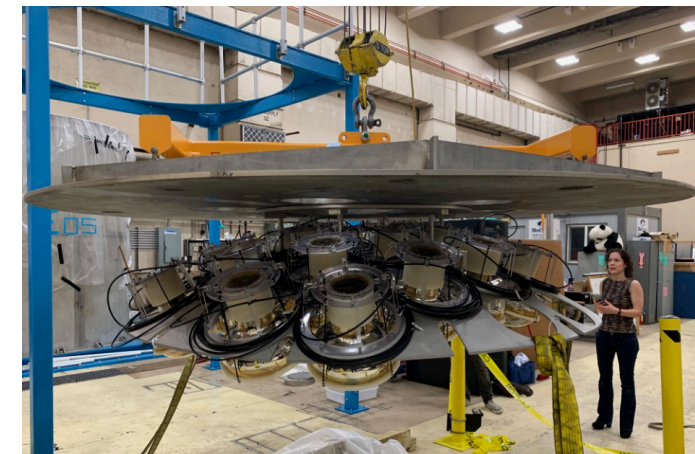
Upper PMT Array during mounting on the top lid (October 2023)
