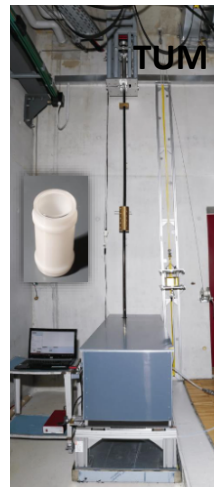
Attenuation Length Measurement Systems ~1% uncertainties up to 50 m @ 430 nm (UC Davis & PALM @ TUM)
