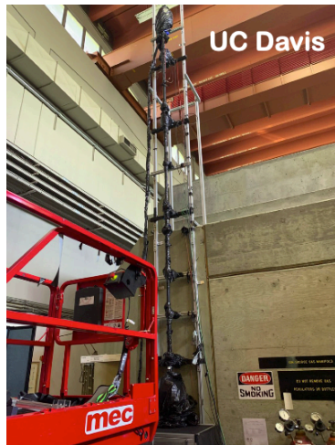
Attenuation Length Measurement Systems ~1% uncertainties up to 50 m @ 430 nm (UC Davis & PALM @ TUM)
