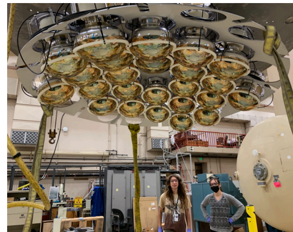
Upper PMT Array during mounting on the top lid (October 2023)
