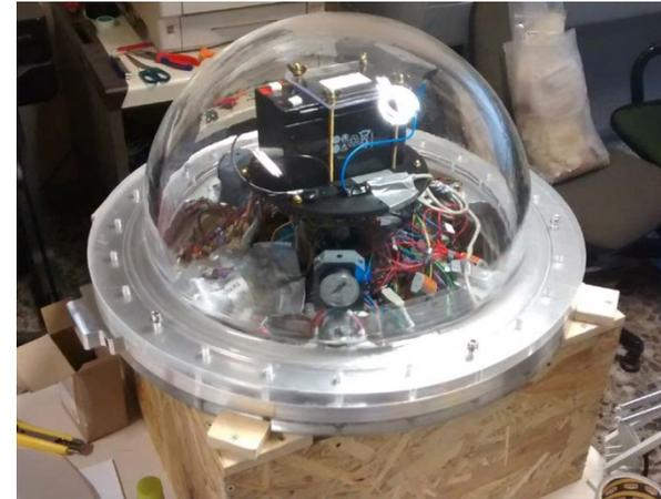
**15mm and 20mm-thick vessels tested
