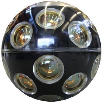
Photodetectors and electronics are arranged inside a pressure resistant vessel
