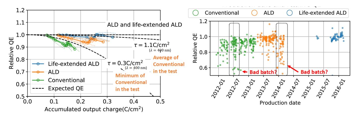
The accumulated charge up to now is only 0.2-0.4 C/cm<sup>2</sup> From the preliminary results lifetimes look like lower than expected. One possible explanation can be the presence of bad batches.
