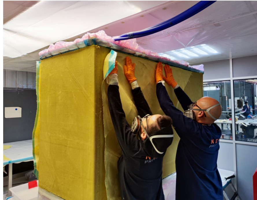
Placing 1 st Twaron layer
