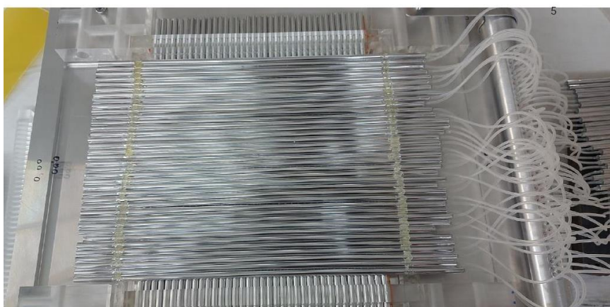
Gluing of the first Y layer and preparation for the second Y layer
