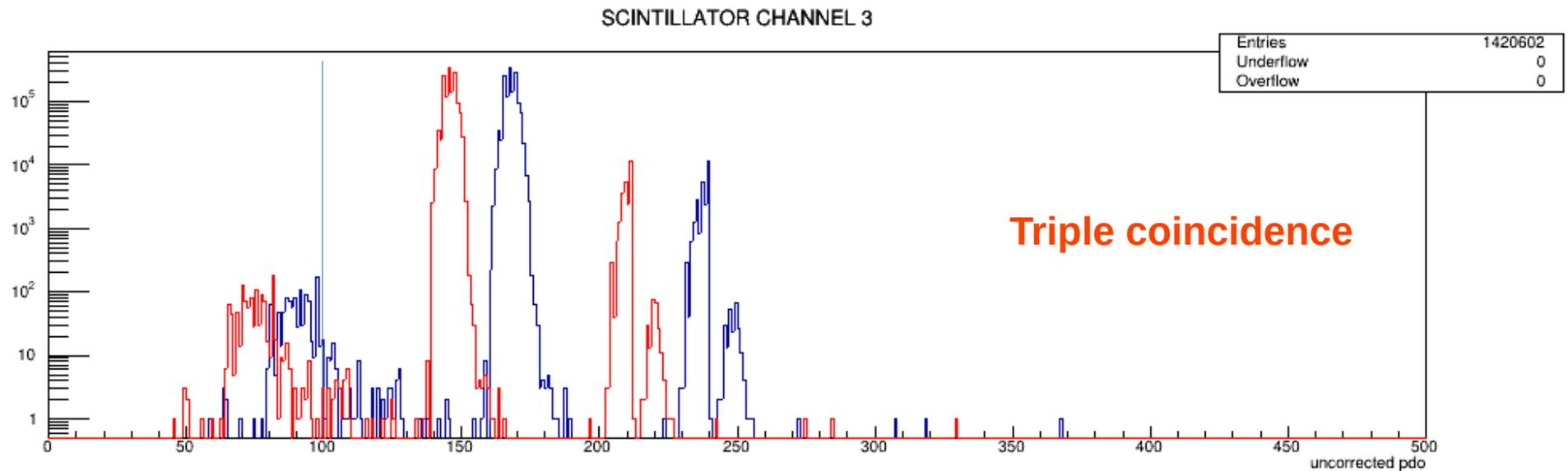
Calibration function is a first order polynomial using the ADC observed range
