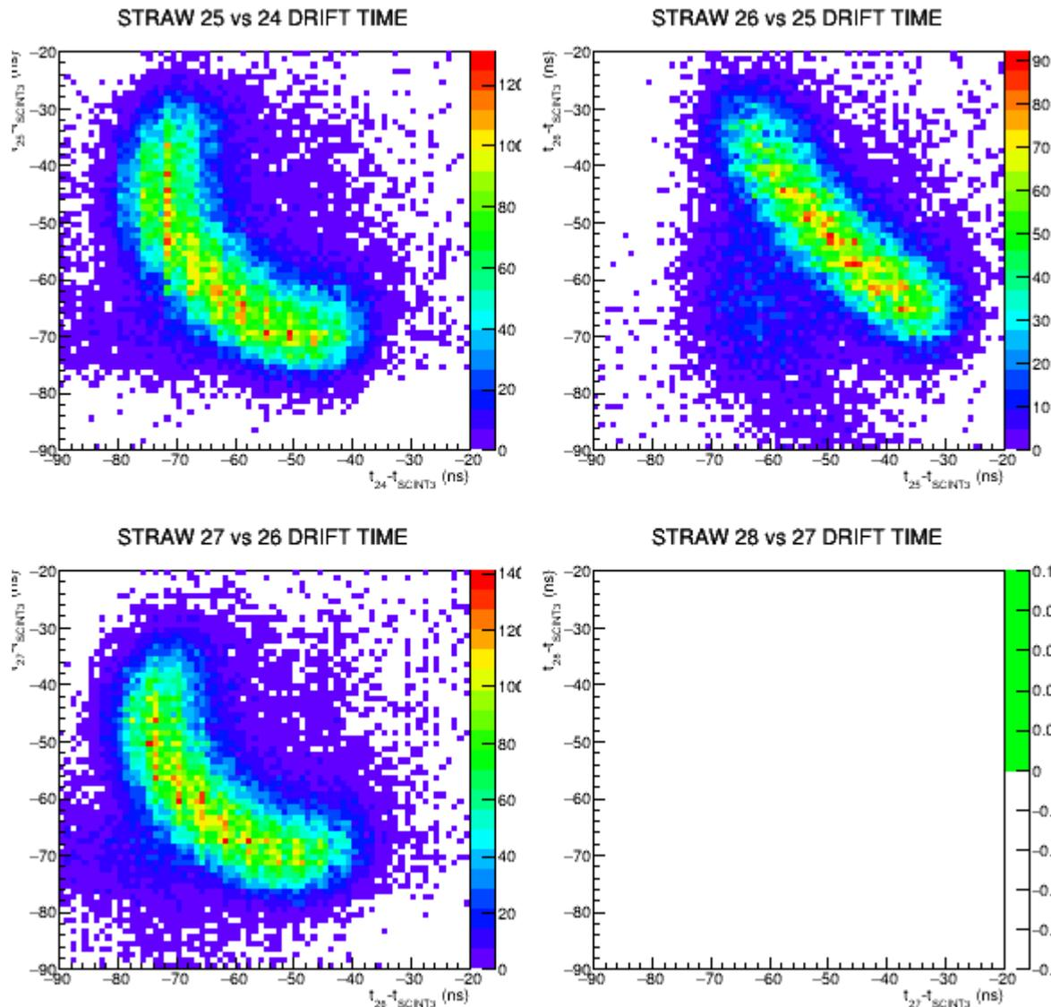
**Drift time** is obtained by subtracting the straw calibrated time and the scintillator coincidence calibrated time
