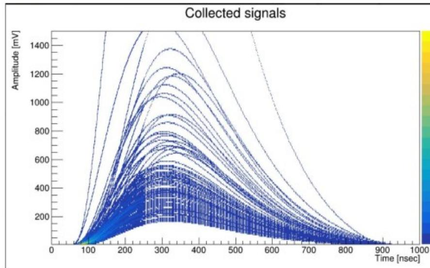
LTSpice amplifier & shaper response to the signals provided by Garfield
