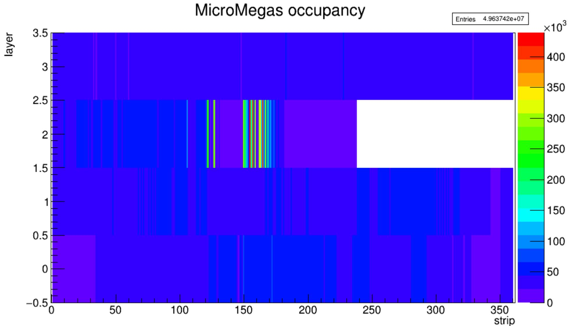
LAYER 2, that is the one read by both Mu2e and APV board, shows problematic strips:
