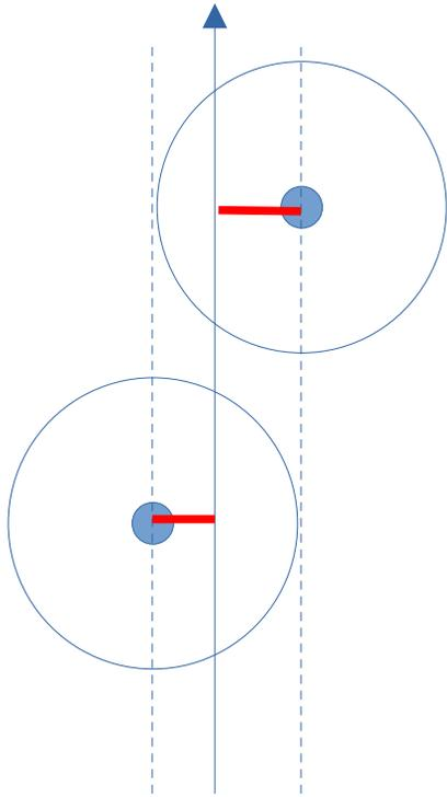
If we consider the beam perpendicular (in fact we know it a sigma of  $\sim 2.6^\circ$ ) the **sum of the drift distances** is **constant** (= the x distance between the wires)!
