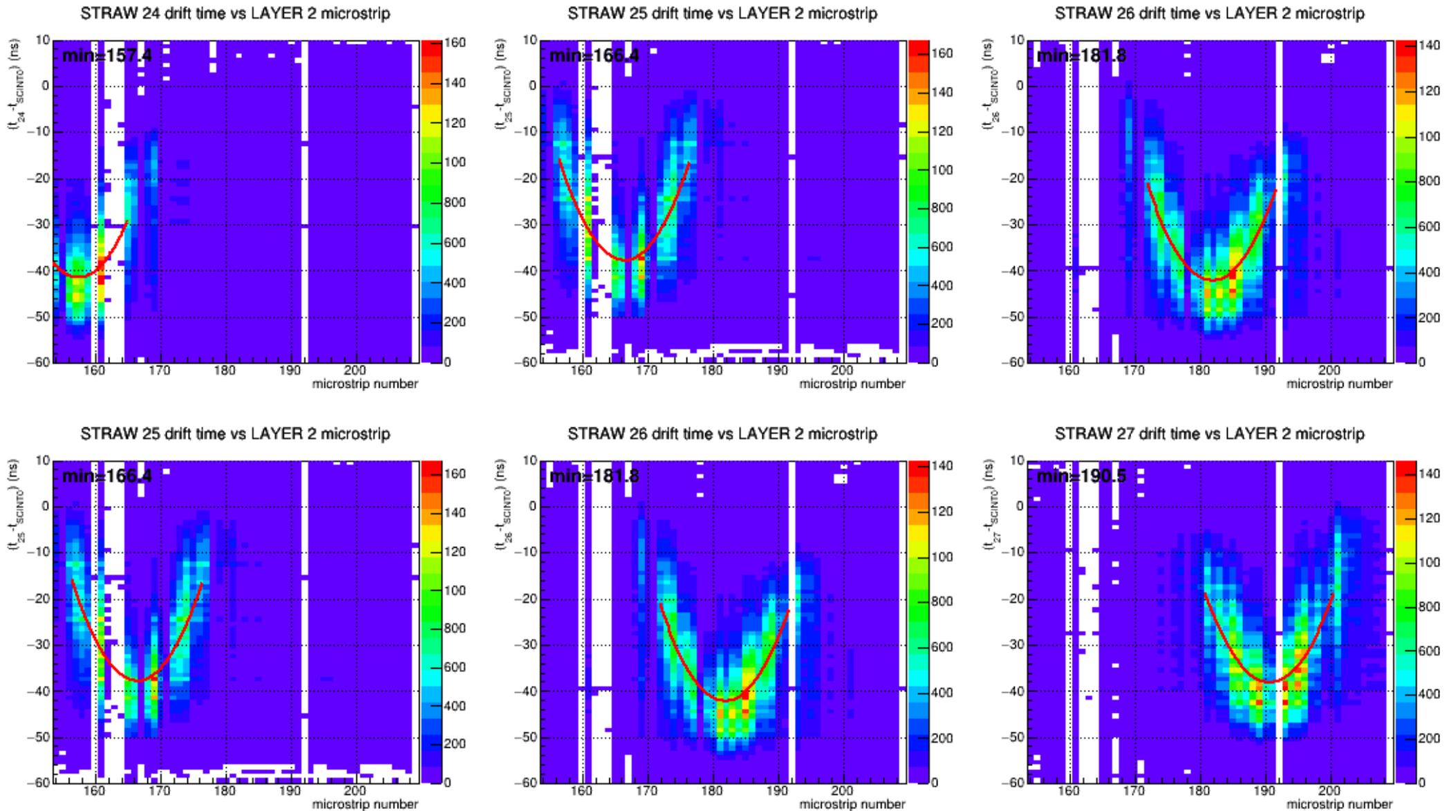
One entry per microstrip hit (not for cluster). Parabolic fit. 1 strip=250  $\mu\text{m}$
