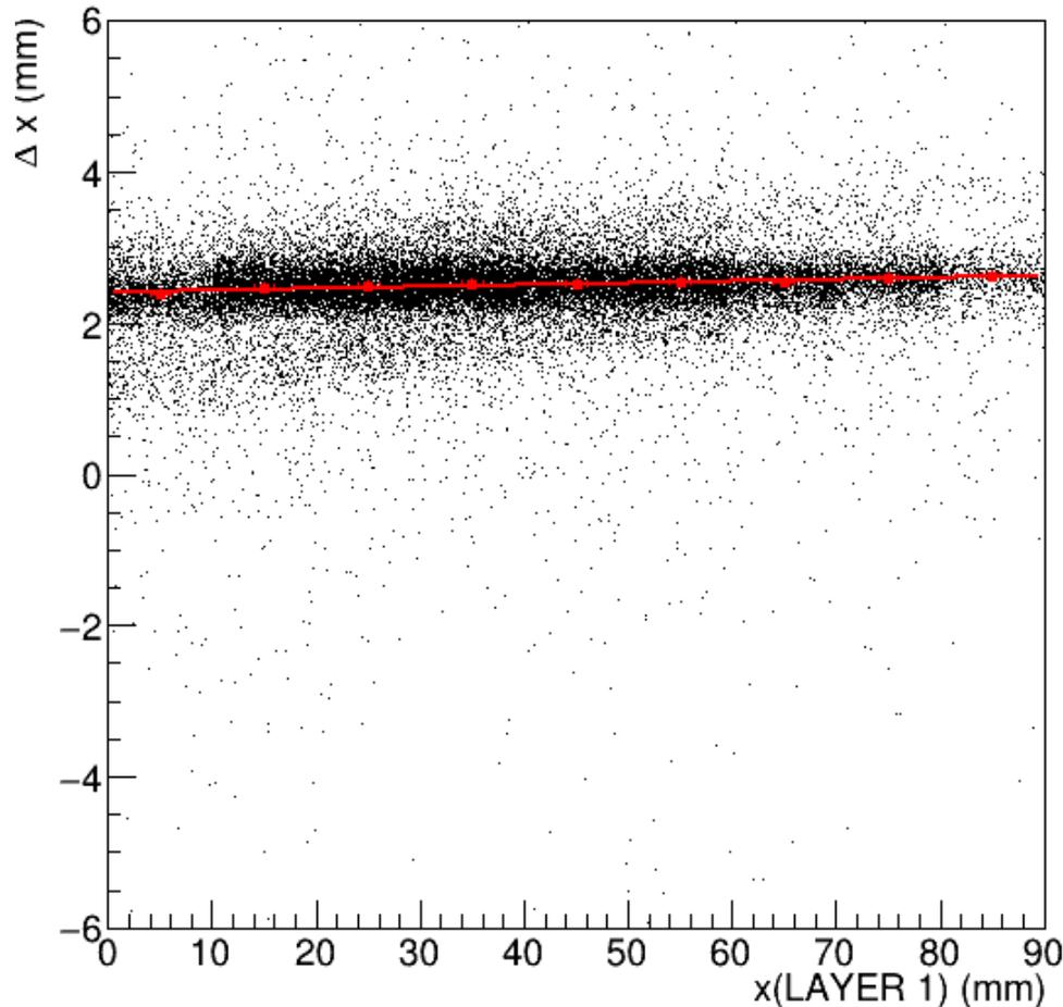
The coordinate  $x$  is given by the strip number multiplied by the  $250 \mu\text{m}$  pitch.
