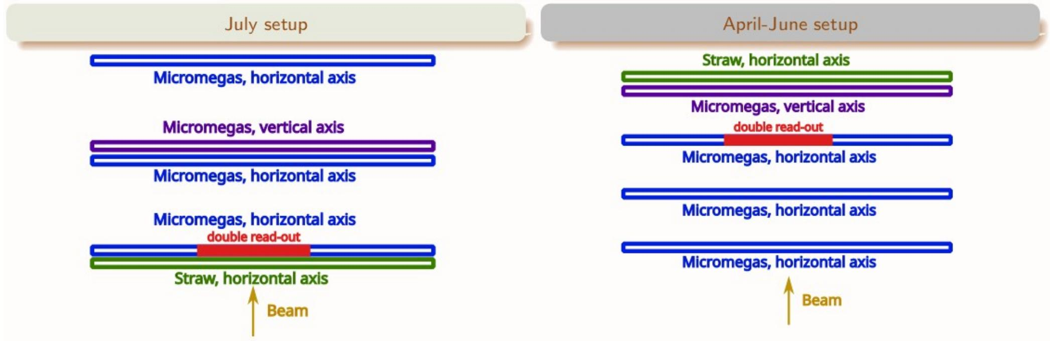
Now the MicroMega close to the straw can be used to fit the track (no extrapolation errors)
