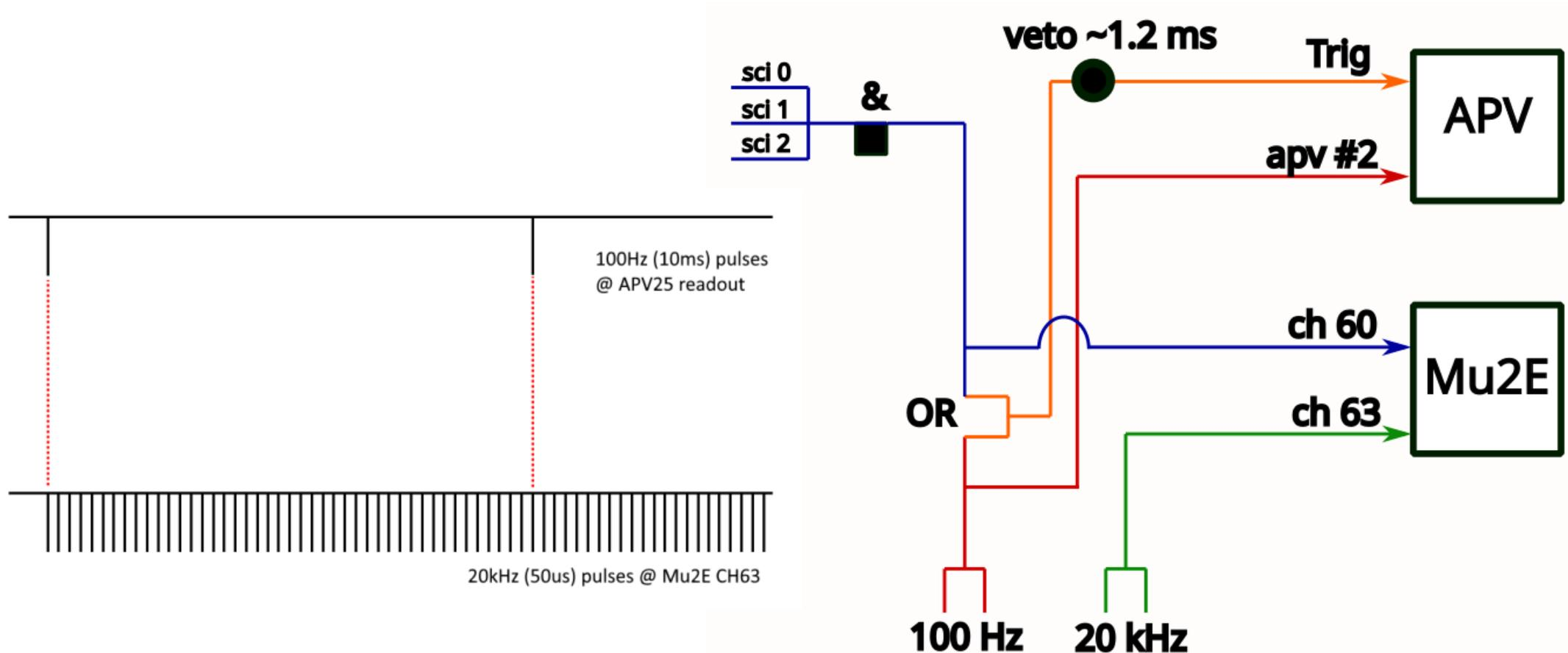
The same pulse generator sends a signal with period  $50 \mu\text{s}$  to the VMM board and 10 ms to the APV boards.
