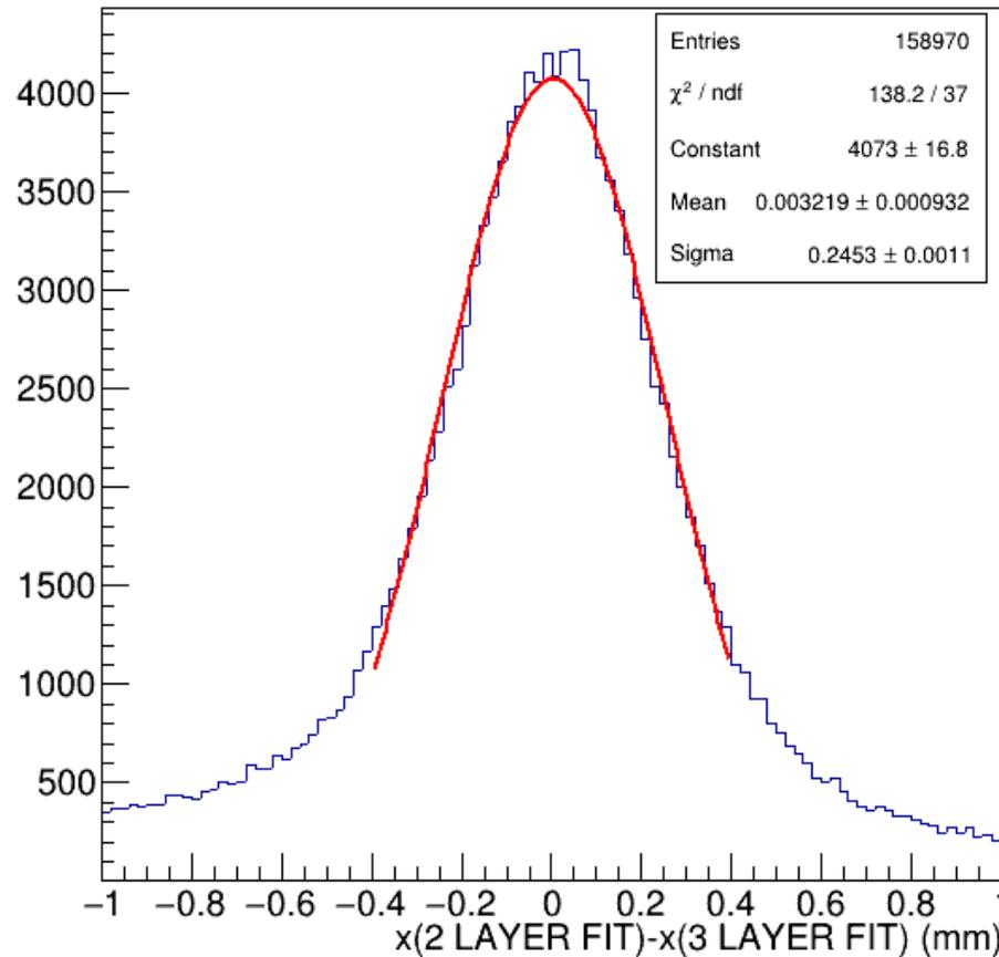
The pointing resolution obtained using LAYER 0 and 1 only is  $\sim 250 \mu\text{m}$
