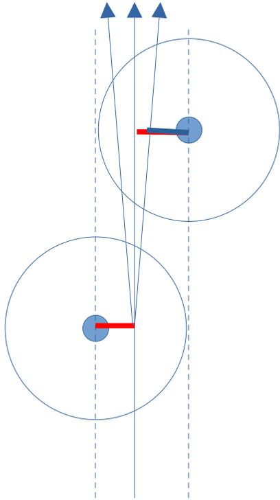
In fact the beam is not exactly perpendicular: there's a sigma of  $\sim 2^\circ$  on the angle that corresponds to  **$\sim 250 \mu\text{m}$**  on 7 mm.
