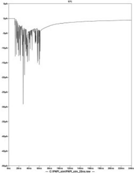
Garfield simulated signal from straw tube
