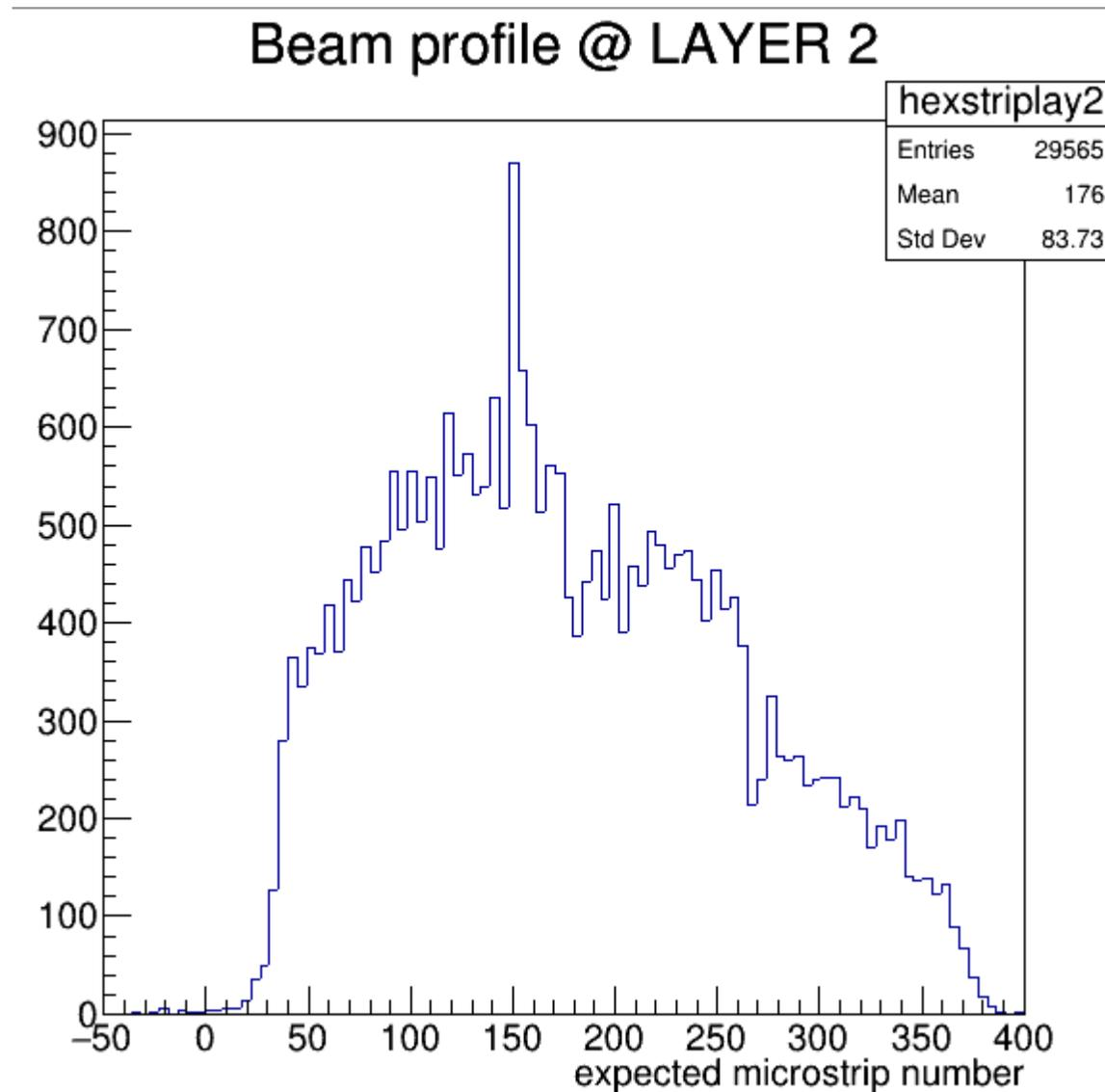
The expected strip obtained by the intersection of the LAYER 1-0 track with LAYER 2 can be used to select the correct cluster on LAYER 2
