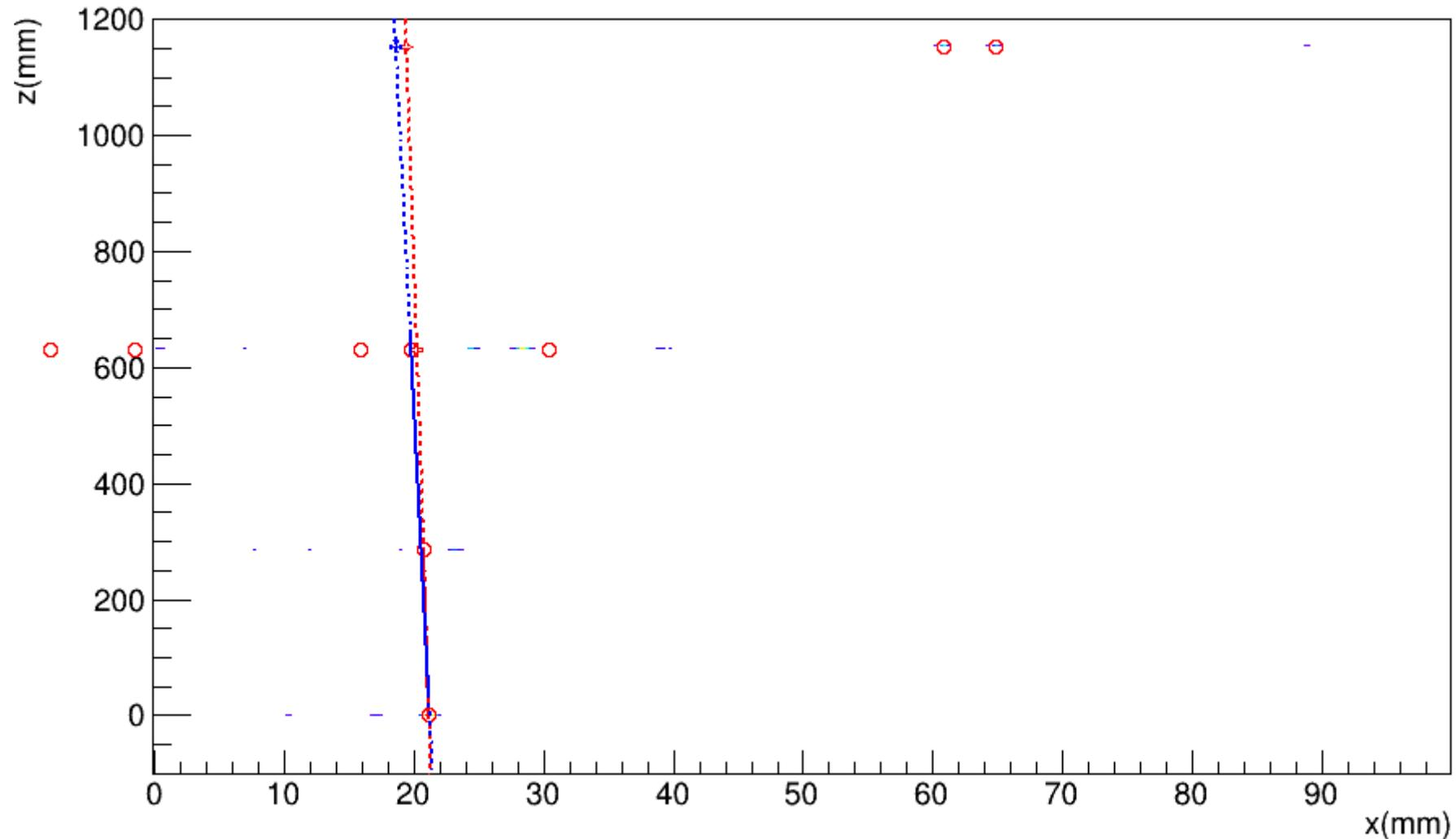
Compare the extrapolation to the straw layers using LAYER 0&1 fit with the one obtained fitting LAYER 0&1&2 when LAYER 2 cluster center is within 1 mm from LAYER 1-0 track
