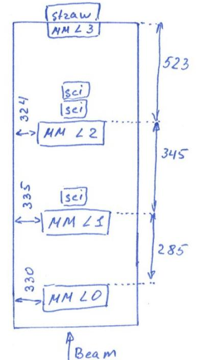
4 MicroMega layers (first 3 with vertical strips, last with horizontal strips)
