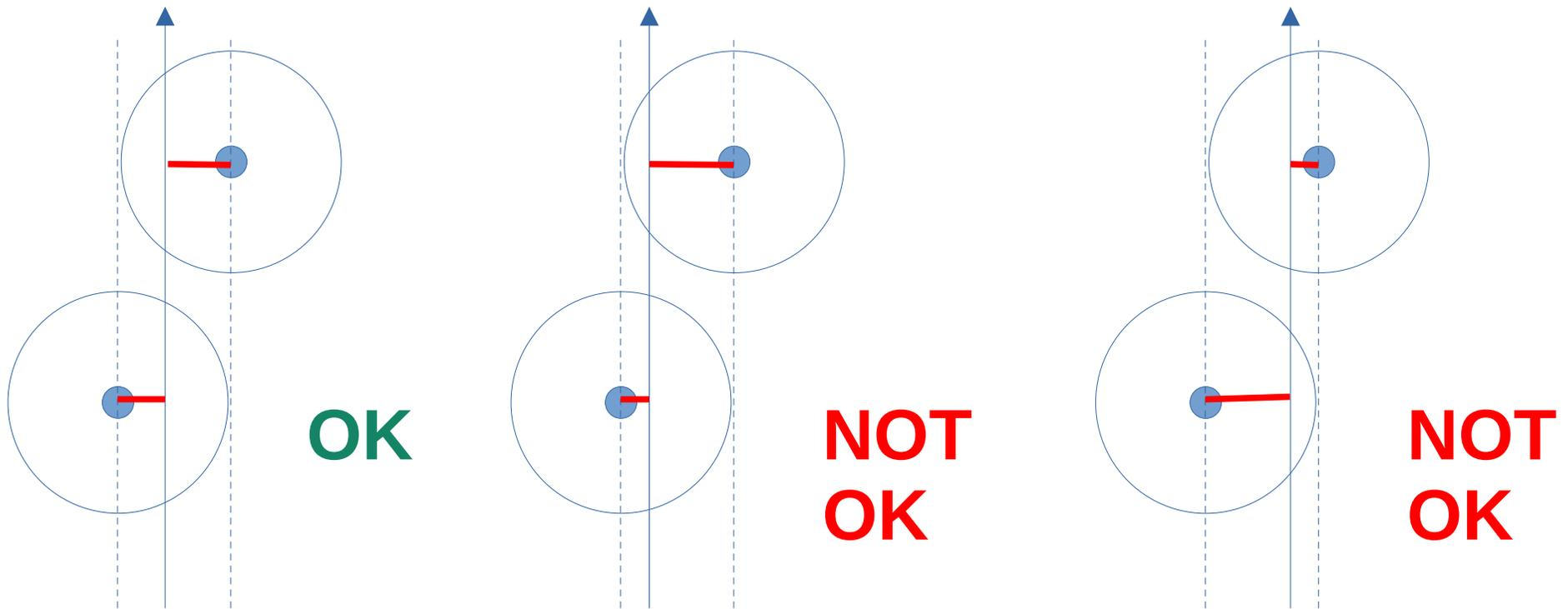
The condition to be far from the wires can be checked looking at the “**drift time asymmetry**” between the straws: the difference between their drift times is 0 when we are far from both wires, different from 0 otherwise.
