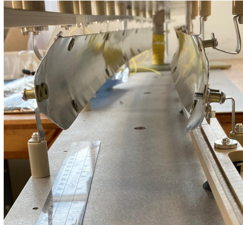
A mockup of the kicker cage, used for tests and practice measurements.
