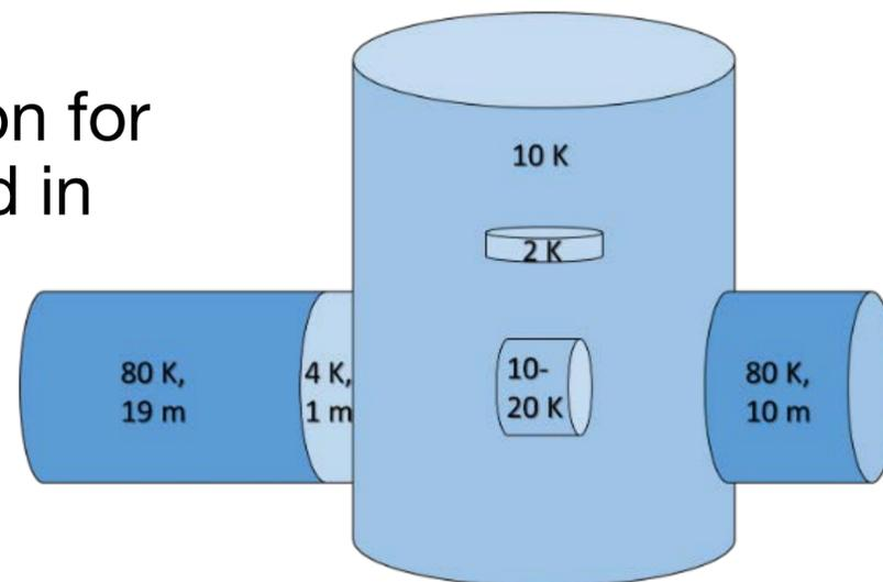
**Source:** S. Hanke, K. Battes, X. Luo and C. Day: Cryopumps at the extremities of the beampipes: design and performance. Beampipes for Gravitational Wave Telescopes 2023, CERN, March 2023, <https://indico.cern.ch/event/1208957/>
