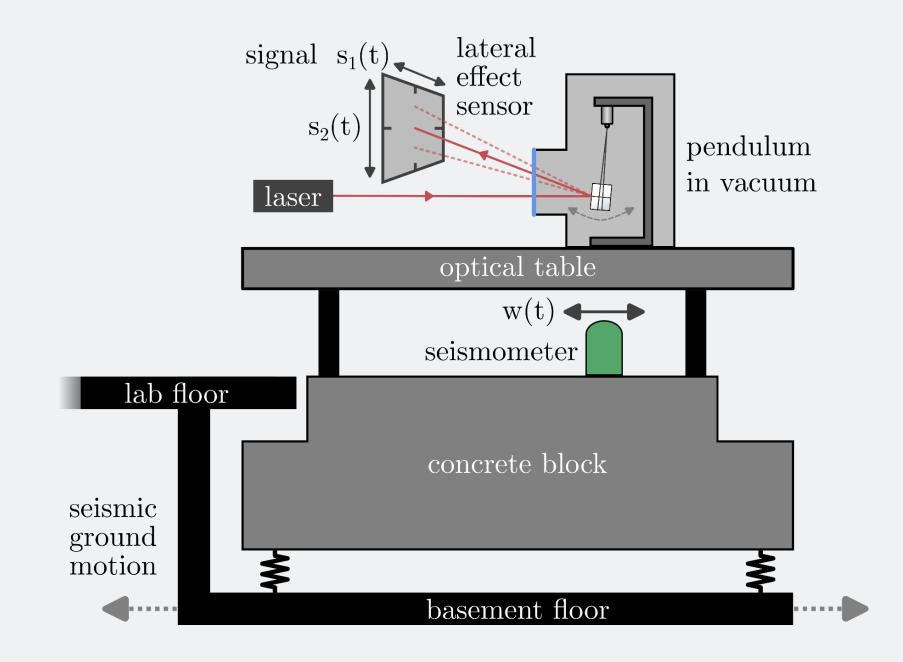
The test-mass with a weight of 100 g has a rectangular profile to provide sharp contact points to the suspension wires. Q-factors between  $10^4$  and  $10^5$  were observed for the suspension modes. The horizontal deflection of the beam  $\phi_1$  mainly corresponds to excitation of the yaw mode resonance around 3 Hz while the vertical deflection  $\phi_2$  is dominated by the main pendulum and pitch-mode at 1.4 and 10 Hz, respectively.
