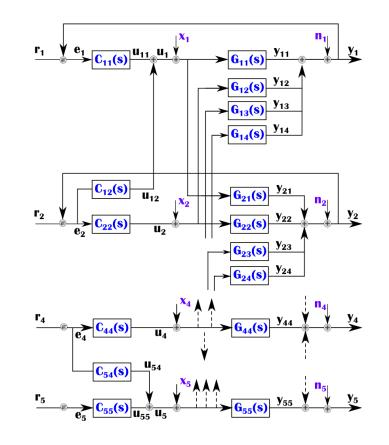
We have represented the interferometer configuration for 04 as an optical plant of 5 cross-coupled longitudinal DoFs with sensors, inputs, outputs, drivers, controllers and actuators <u>matrices</u> with a MIMO scheme.
