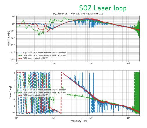
Green plot: OLTF reconstructed using this MIMO approach. Blue plot: OLTF obtained using the usual SISO approach. Red plot: Equivalent OLTF. Using the usual OLTF estimation approach one is taking into account the couplings among the loops.
