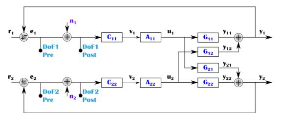
Scheme for a control matrix 'C', an actuator matrix 'A' and an optical plant matrix 'G'.
