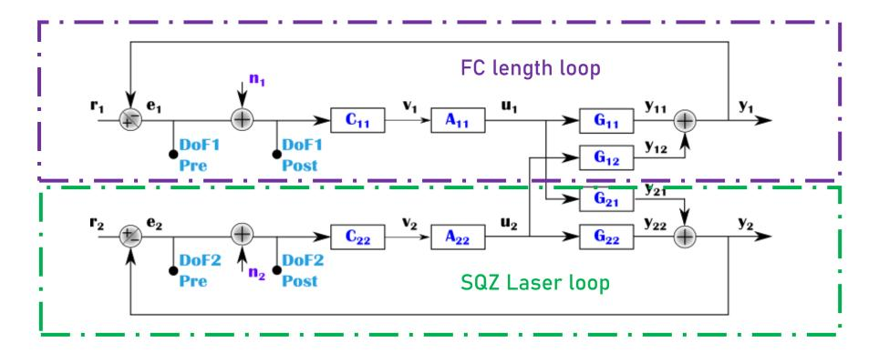
First, using a proper MIMO system identification approach we aim to understand the full TF matrix of the optical plant "G(s)". Secondly, since the system exhibits strong cross-coupling terms, one should use a MIMO system control strategy.
