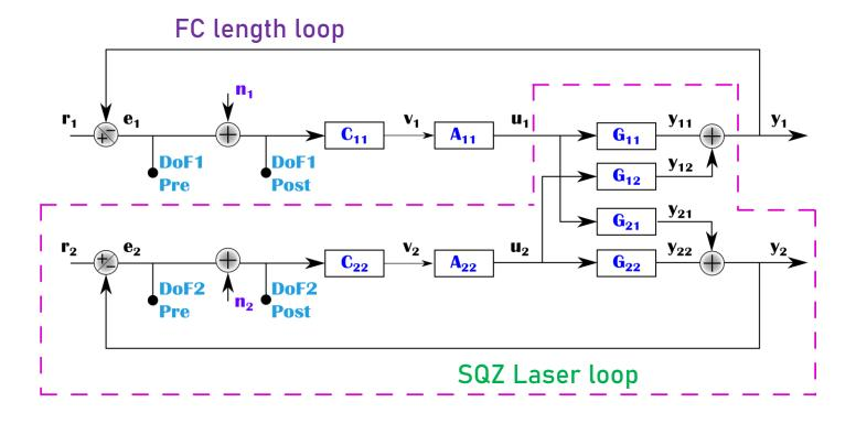
Because with this method one can not decouple the effects of the two closed loops in the estimation of the OLTFs of the system.
