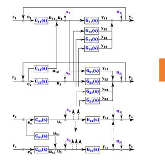
To represent the interferometer in a MIMO scheme, one has to define the matrices D, H(s), A(s), O, B(s), C(s), I and G(s). These are  $p \times q \times n$  dimensional matrices. Where p is the number of inputs, q number of outputs and n is the length of the frequency vector.
