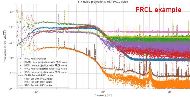
Blue curve is the PRCL noise injected. Dashed plots are the spectra of the longitudinal DoFs when the noise of PRCL is injected. Dot plots are the longitudinal noise projections of the PRCL noise on the different DoFs error signals.
