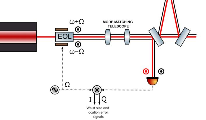
We can then use the same photodiode of the Pound-Drever-Hall error signal to record the beating between the LG10 carrier and the LG10 reflected sideband. Demodulating this signal with I/Q demodulation allow us to obtain two signals containing  $\gamma$  and  $\beta$ :
