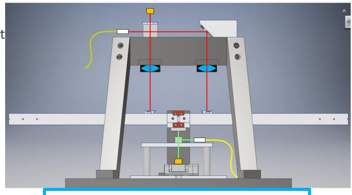
Lenses in the ITF read-out are added to give robustness against static arm tilts
