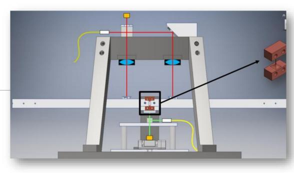
Tiltmeter arm is suspended through **Cu-Be flexible**joints, 100μm x 500μm in section, very similar in design
