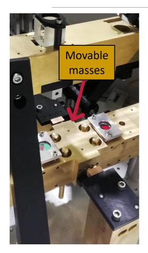
The center of mass was raised by about 35  $\mu$ m to reduce its distance from the bending point and therefore reduce the seism-to-tilt coupling. Resonance frequency changed from 23 mHz to 12 mHz
