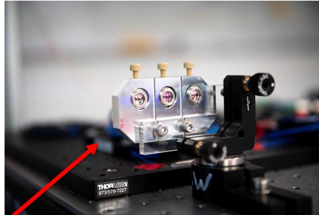
Fibre collimator/partial reflectors
