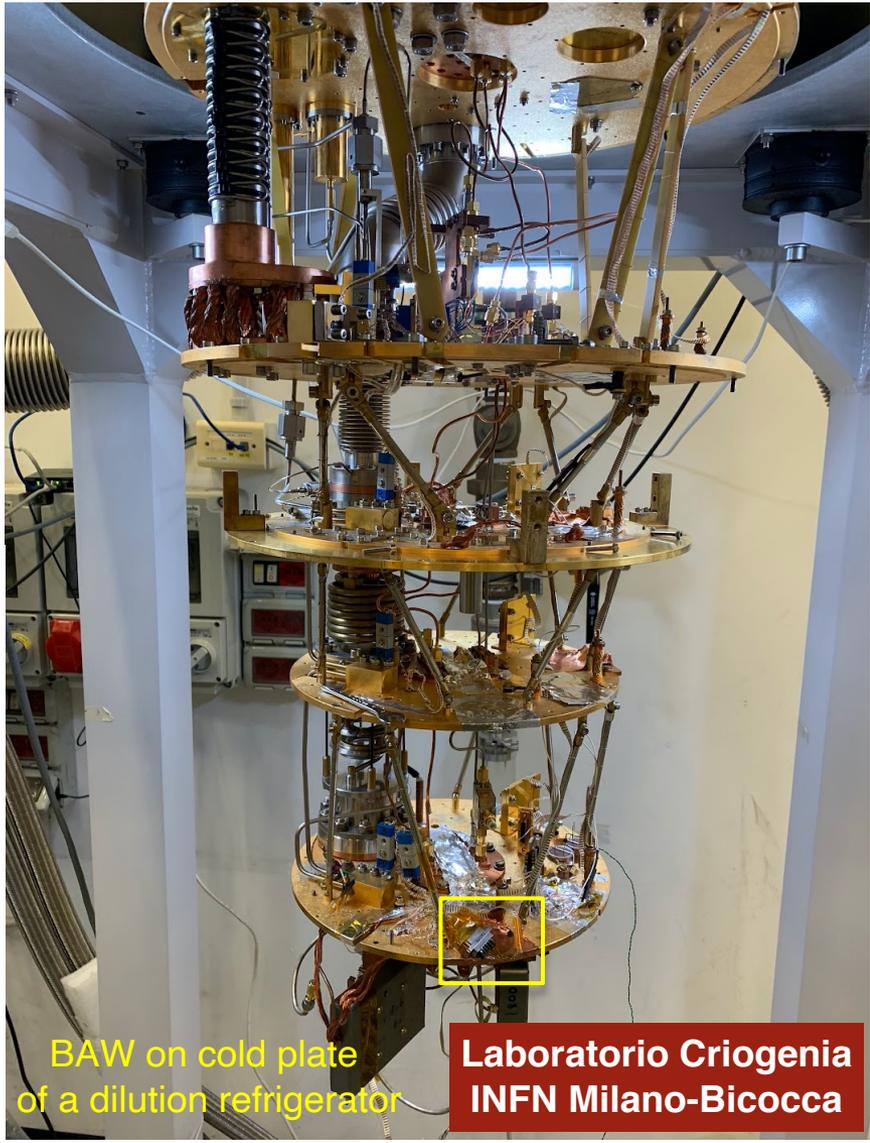
BAW on cold plate of a dilution refrigerator
