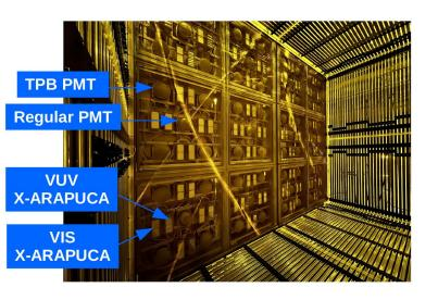
Liquid argon is a scintillator. VUV photons are emitted when a charged particle excites the argon.
