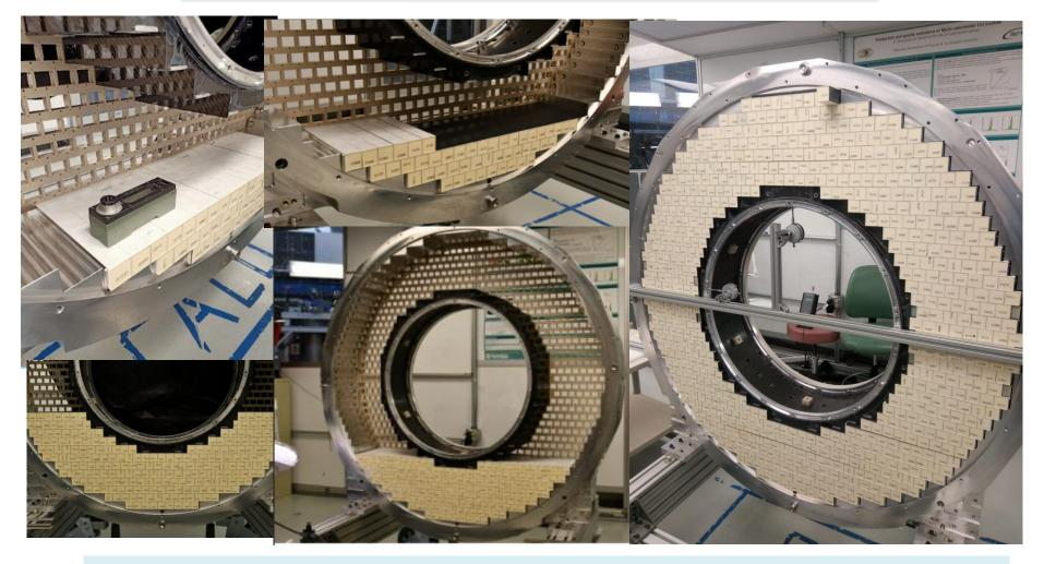
Successful outgassing of all 674 crystals selected for optimized positioning on the disk + great stacking of all crystals on mechanical support
