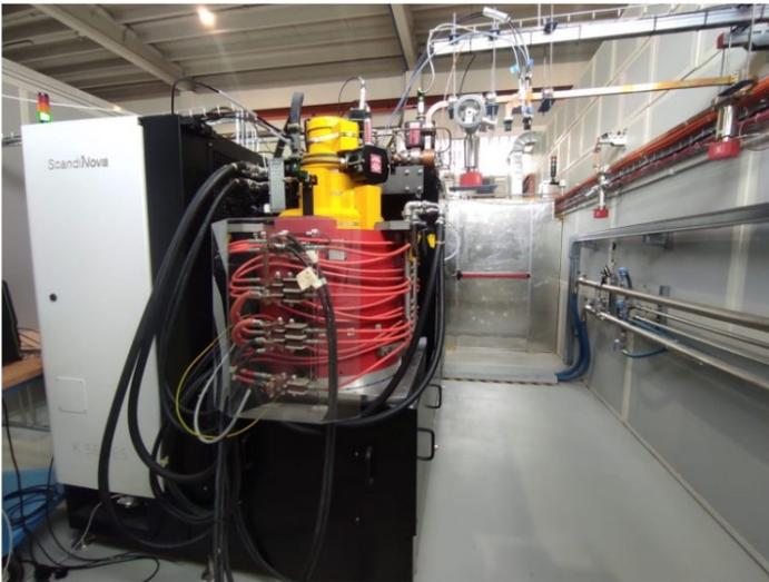
**TEX** (TEst stand for X-band) is the new infrastructure at LNF, co-funded by the **LATINO** project, devoted to the radiofrequency (RF) in X-band and, in general, to the development of all the technologies and systems related to a particle accelerator.
