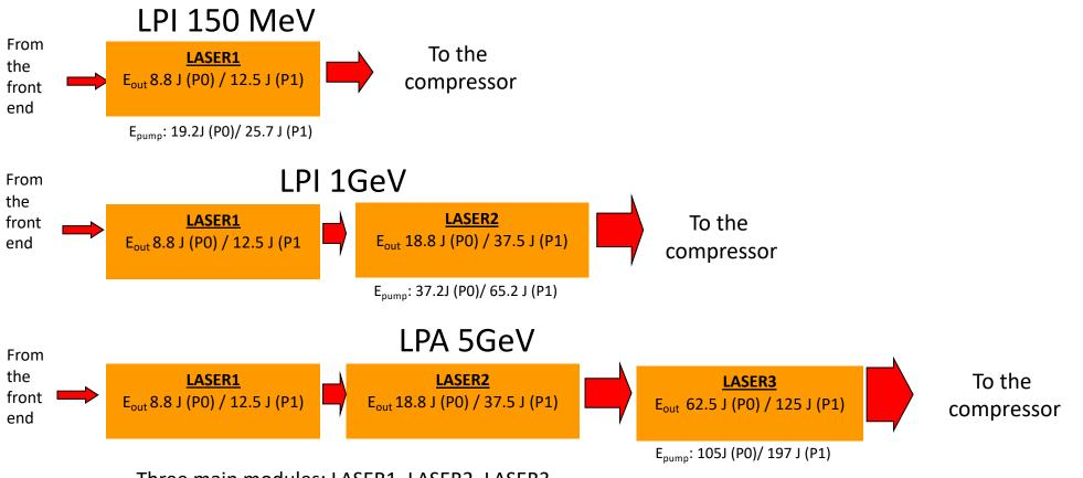
Three main modules: LASER1, LASER2, LASER3 LASER1: stand-alone for LPI 150 MeV
