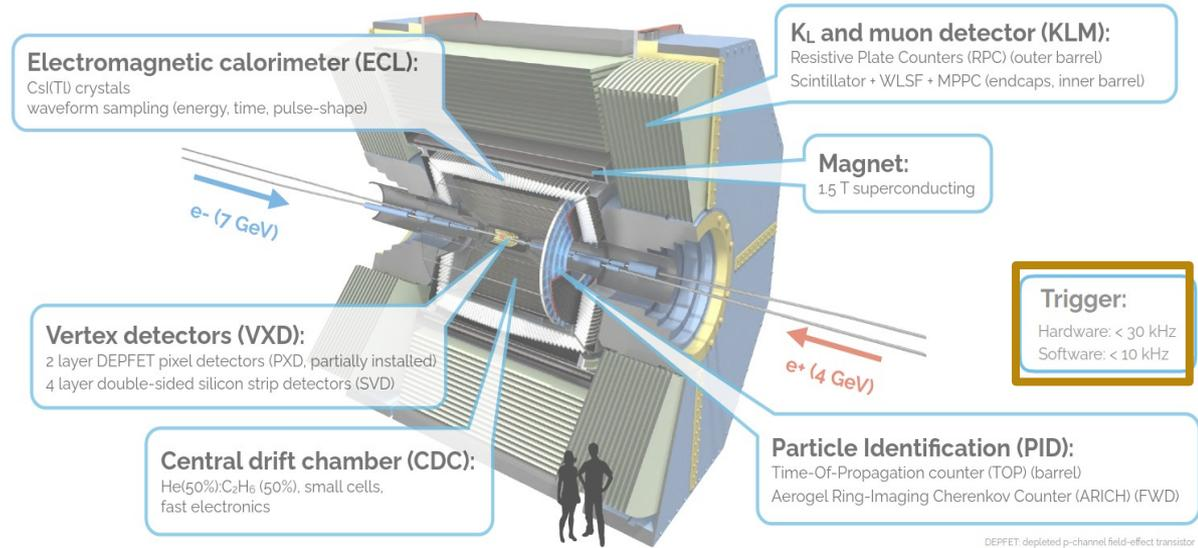
DEPFET: depleted p-channel field-effect transistor
