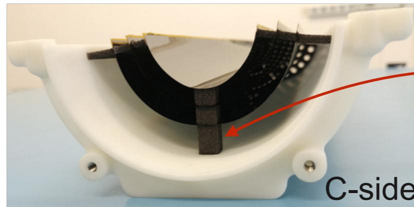
Wedges replaced with half-ring due to excessive deformation from cylindrical shape
