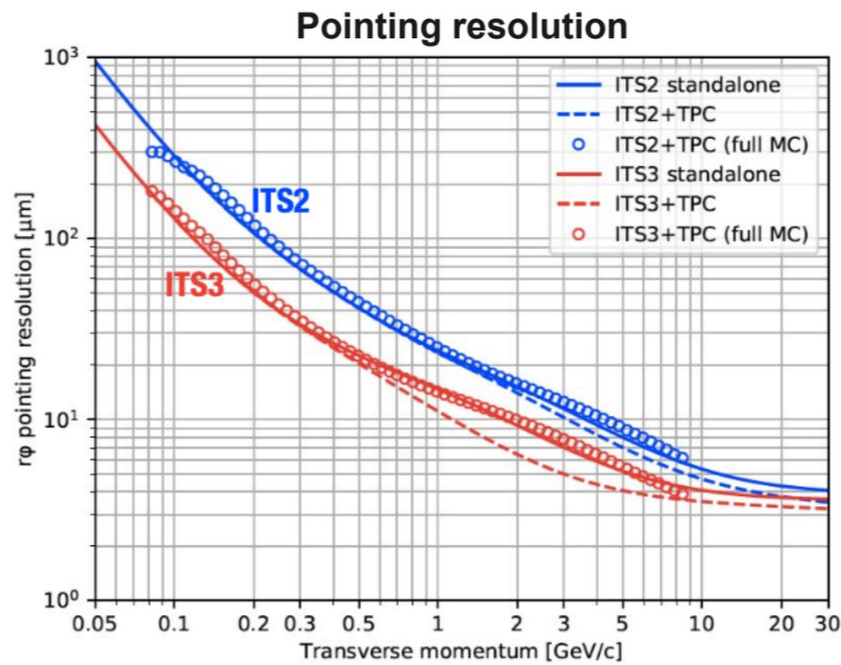
Improved pointing resolution and tracking efficiency for low momenta ( $\times 2$  at all  $p_T$ )
