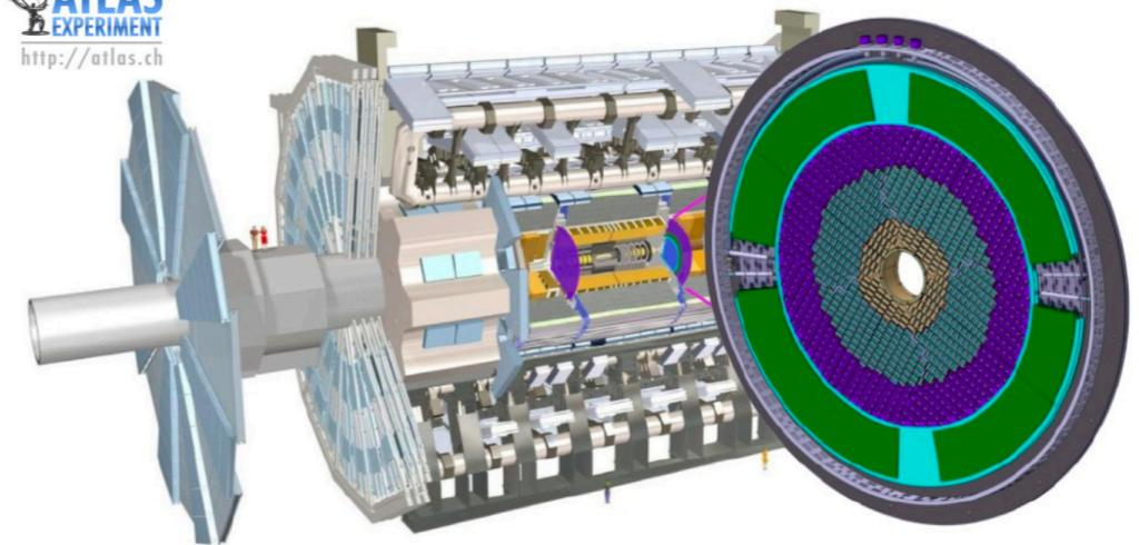
ATLAS High Granularity Timing Detector (HGTD)
