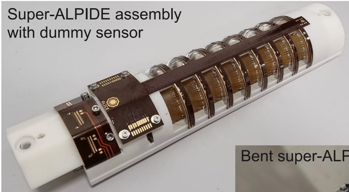
Bent super-ALPIDE sensor under test
