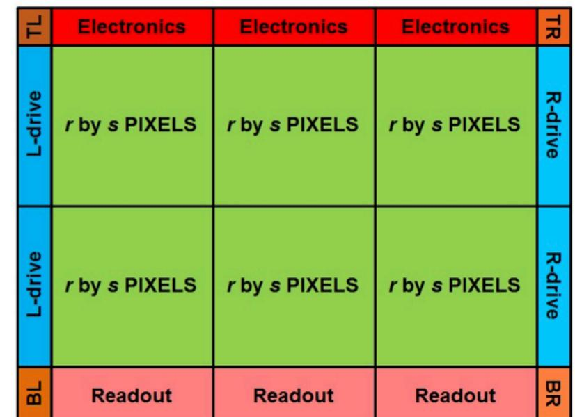
Extending the size of the sensor beyond the reticle field of view
