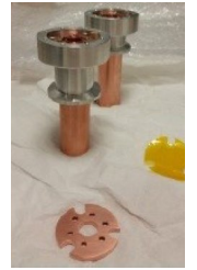
Injection and extraction flanges with horn-antennas
