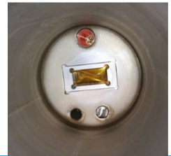
Injection and extraction flanges with horn-antennas
