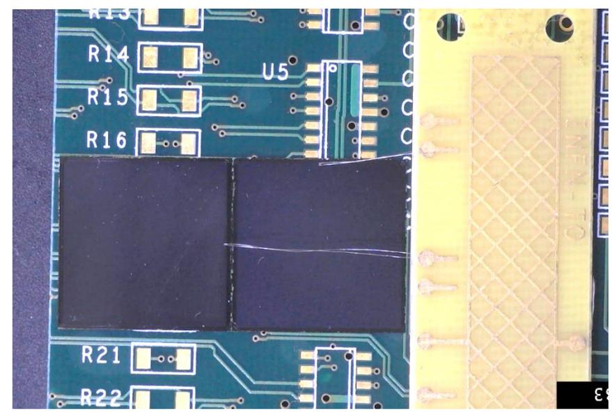
Long wire bonding (performed at INFN-To)
