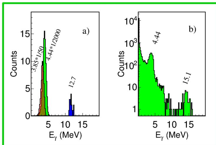
Gamma-particle coincidences are a powerful tool for the investigation of different topics as observed in experiments performed by using the CsI(Tl) crystals of the CHIMERA device. Currently the gamma detection threshold is around 1.5 MeV.
